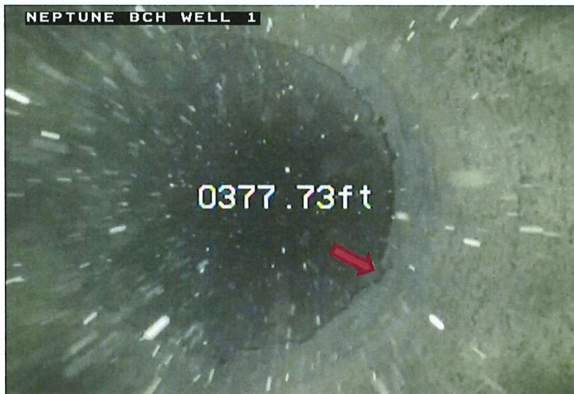
Photograph 4 - Bottom of Casing Looking Down
