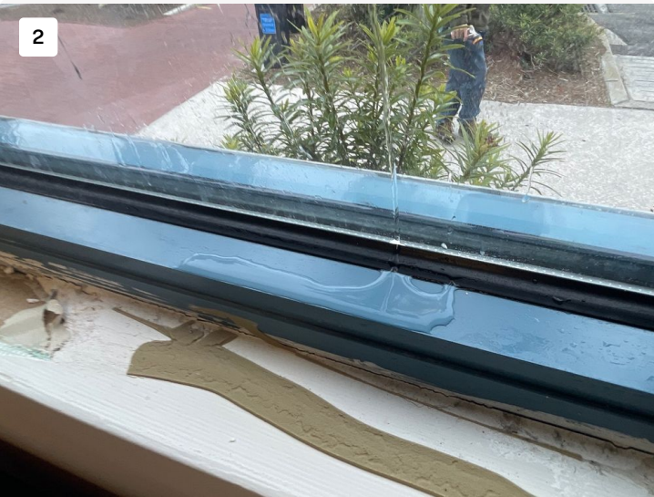
Water test showing water intrusion at windows around window seals and mullion entry points
