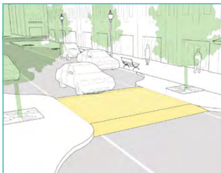
8. Speed Tables/Elevated Crosswalks
