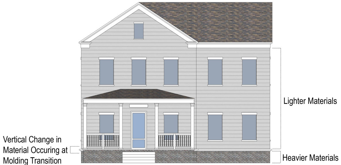
Figure 27-24-31: Residential building material and details
